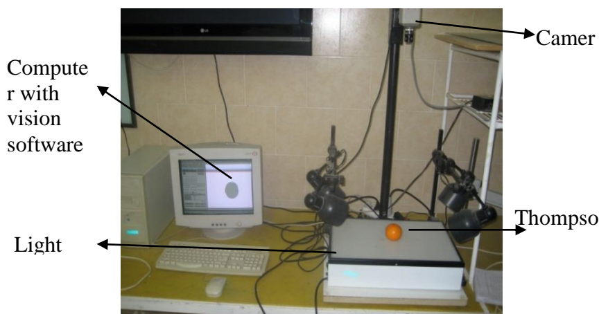
Figure 1 - Experimental setup of the mass estimation software.
